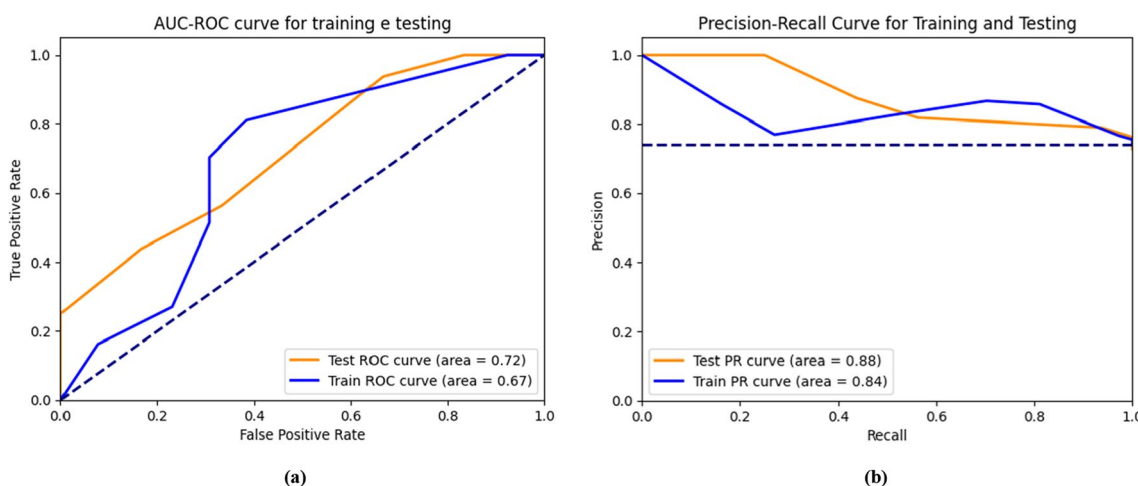
Fig. 2 Visual comparison of a performance model for training and testing set for Random Forest. The blue lines represent the training curves, the orange lines represent the testing curve, and the dashed lines of a random classifier. A higher curve represents a better performance of the model, to be acceptable it must exceed the dotted lines. The first figure represents the AUC-ROC curve (a). The AUC-ROC curve shows the relationship between the true positive rate and the false positive rate. The second figure represents the Precision-Recall (PR) curve (b). The PR curve shows the relationship between precision and recall. AUC-ROC = Area Under the Curve—Receiver Operating Characteristic
