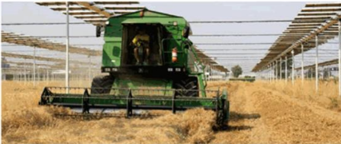
Figure 3 Panels mounted on double-axis trackers are kept horizontal to enable cereal harvesting with a conventional combine harvester (Courtesy RemTec https://remtec.energy/en/agrivoltaico/ )
