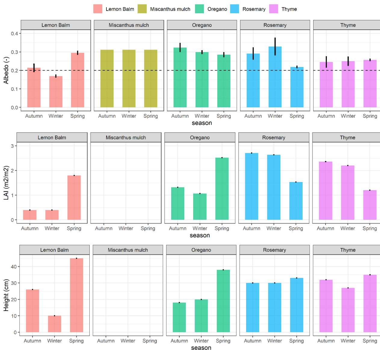
Figure 10 Mean value of Albedo, Height and LAI for the season considered. The dotted lines represent the albedo value of bare soil (0.21) and Miscanthus mulch had an albedo value of 0.30, both albedo values were assumed for all the three seasons considered.
