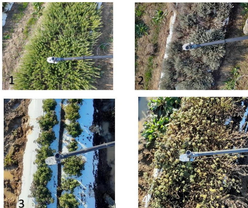
Figure 5 Pyranometers on crops: 1) rosemary 2) thyme 3) oregano 4) lemon balm
