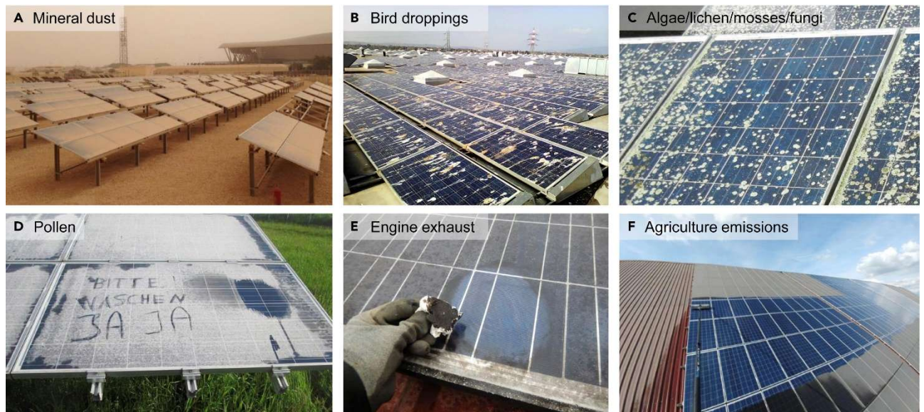
Figure 19. Different sources of particle deposition in utility scale PV system ( Reprinted by [161] With permission of Elsevier ).
