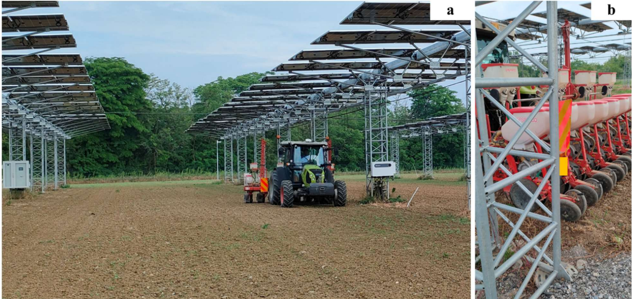
Figure 10. a) Precision seeder in action within the operating space of the APV at Università Cattolica del Sacro Cuore; b) detailed distance between implement and stilt during sowing ( Original photographs taken by the authors at the APV plant of Università Cattolica del Sacro Cuore, Piacenza, Italy ).
