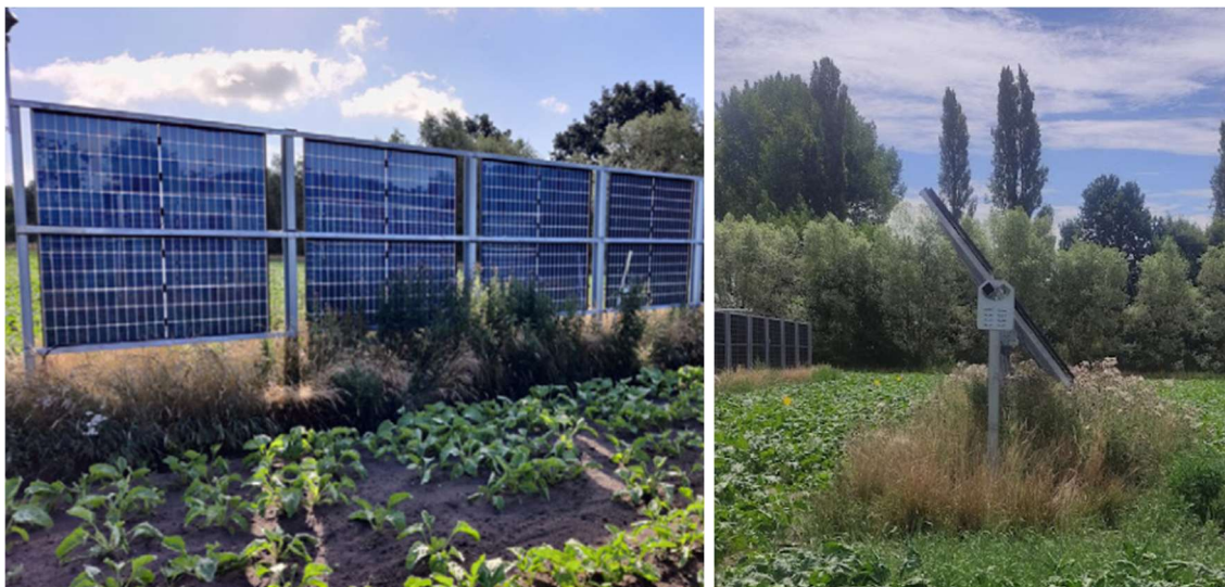
Figure 17. Weeds development in the non-cultivated areas of Vertical APV system (left) and interspaced monoaxial APV system (right) (Reprinted from [17] with permission of Elsevier).
