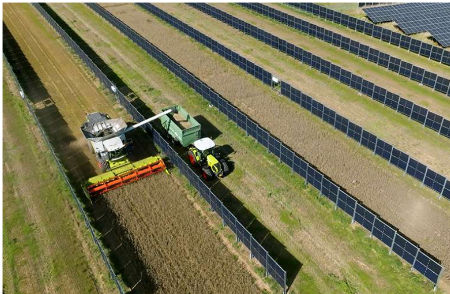
Figure 4. Combine harvester in action with concurrent discharge. The combine harvester in the picture is equipped with a header whose width perfectly matches the available operating space (from Next2sun AG, with permission).
