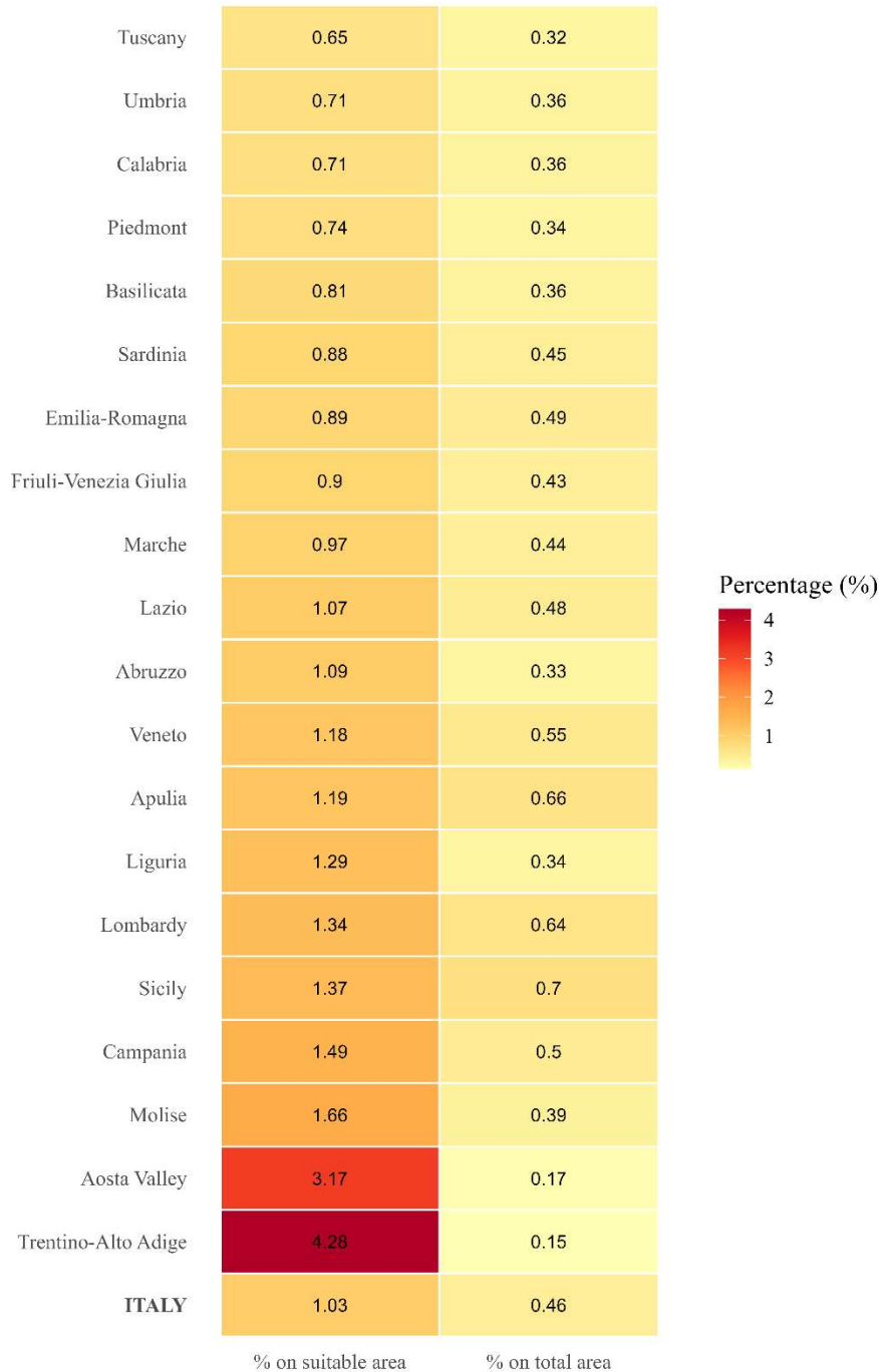
Figure 42. Assumed land requirement (%) to meet the 2030 Burden Sharing targets [1]. The heatmap illustrates the agricultural surface that would need to be allocated to APV systems to meet the renewable energy deployment targets for 2030, assuming a representative APV power density of 0.577 \text{ MW ha}^{-1} . Results are presented using two complementary reference bases: (a) percentage relative to suitable land only, and (b) percentage relative to total regional surface.
