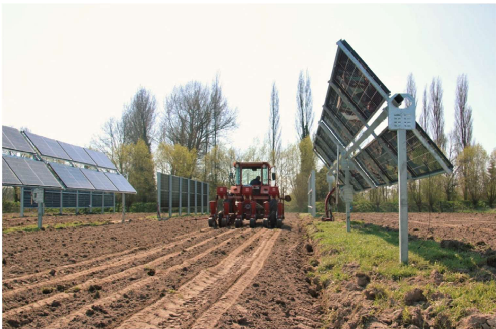
Figure 6. Mechanized cultivation in Belgium. The absence of precision farming GPS guided vehicles forced the operator to maintain the machine at 1 m distance from each side of the APV to avoid collisions ( Reprinted from [17] with permission of Elsevier ).
