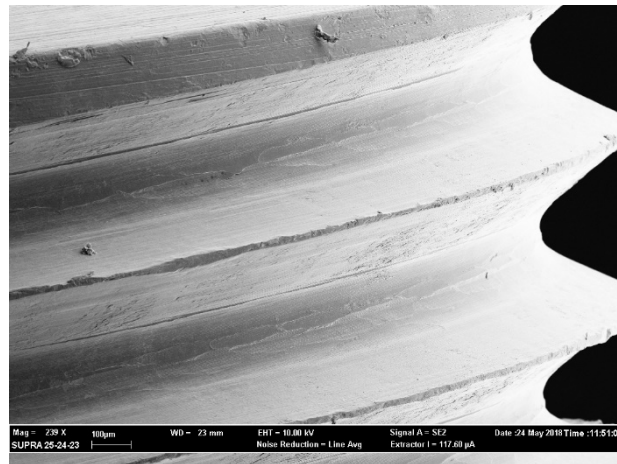
Figure 4. Air polishing and CHX treatment on a machined implant. Magnification 239×.
