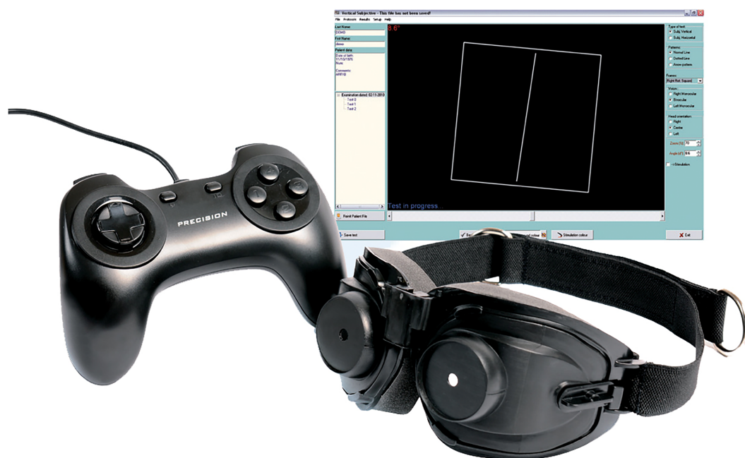
FIGURE 2 Equipment for the SVV/SVH test: the Synapsis ® SVV Software with the stimulus projected at a distance of 2 m, in front of the subject; the contour mask with binocular vision; the joystick used to adjust the line to absolutely vertical and horizontal as perceived by the patient. SVH, subjective visual horizontal; SVV, subjective visual vertical.
