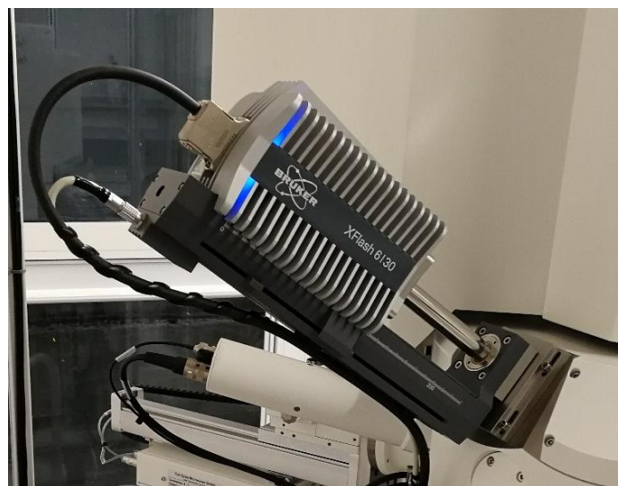
Figure 1.22 Bruker XFlash 6|30 EDX detector mounted on the SEM (Photo by Giulia Papa).
