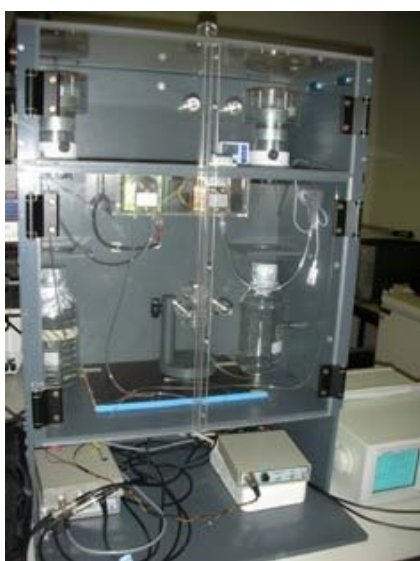
Figure 3. Ussing chamber apparatus used to perform the in vitro trials at the Department of Biosystems, Katholieke Universiteit of Leuven Belgium
