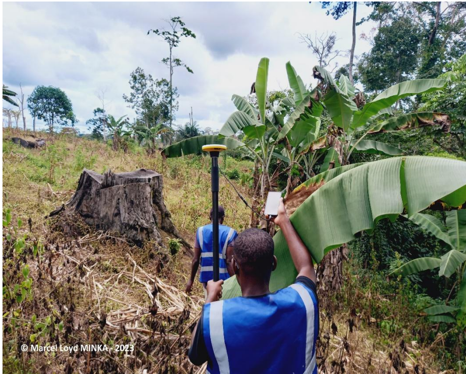
Picture 3: Delimitation of farm limits using Trimble Catalyst DA2
