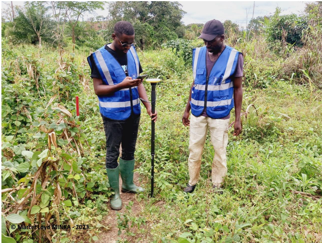
Picture 6: Placing Ground Control Points (GCPs) on each farm corner
