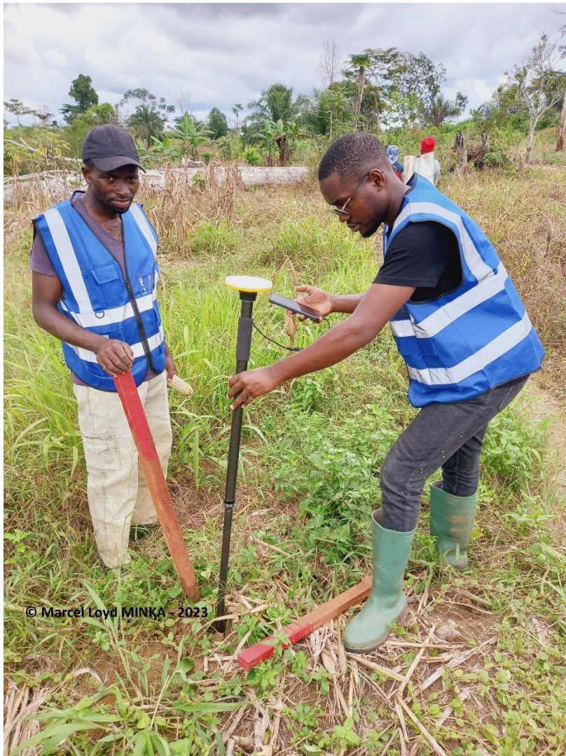
Picture 5: Placing Ground Control Points (GCPs) on each farm corner
