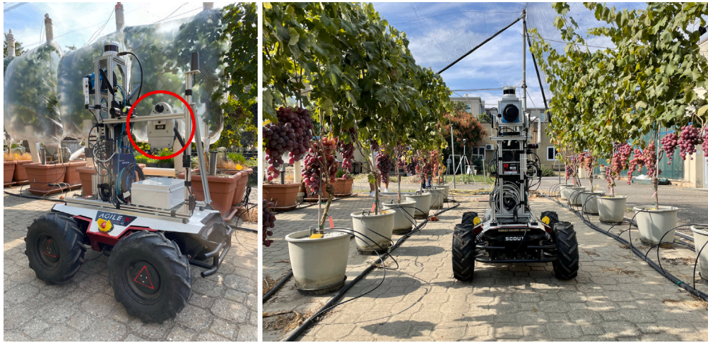
Fig. 2. The robot while acquiring images in the vineyard with the hyperspectral camera mounted on the side. The camera is highlighted with a red circle.
