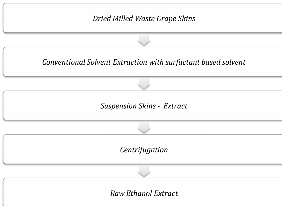
Figure 3.4. Schematic presentation of alternative solvent extraction (Application A of Figure 3.3)
