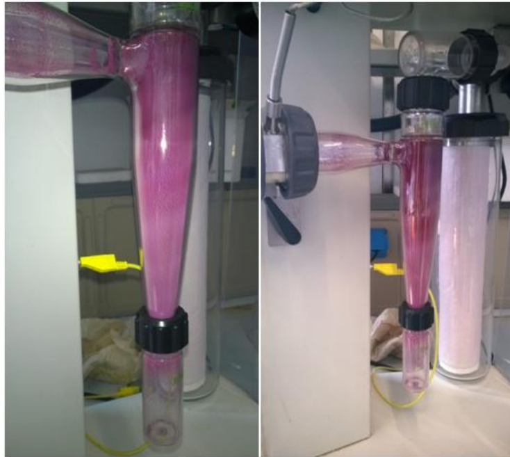
Figure 4.18. Cyclone system at the spray-drying exit for powder collection (trial with Barbera skins extract enriched in Tw20).
