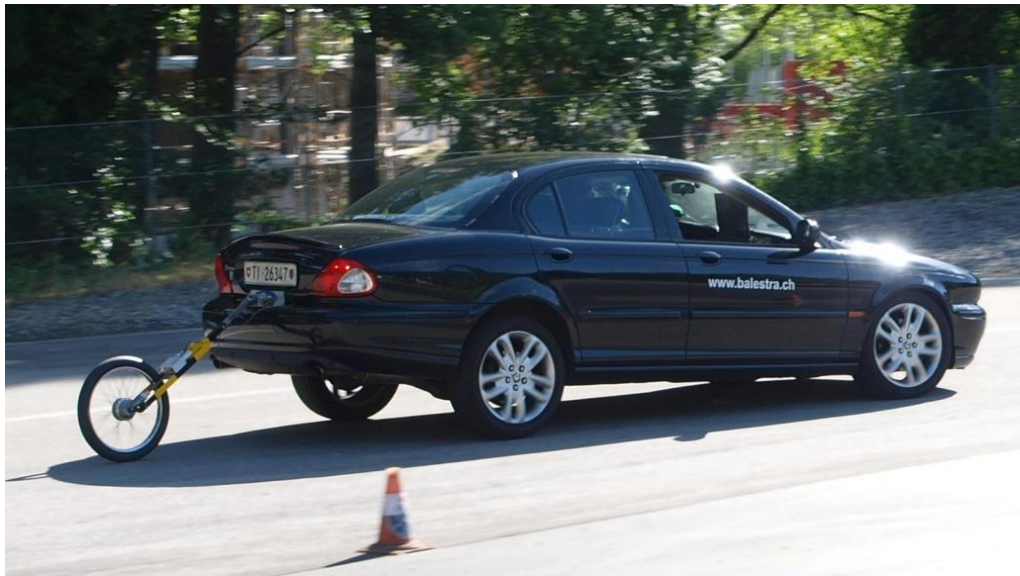
Figure 10. Fifth wheel sensor to record space/speed (© Ing. M. Balestra)
