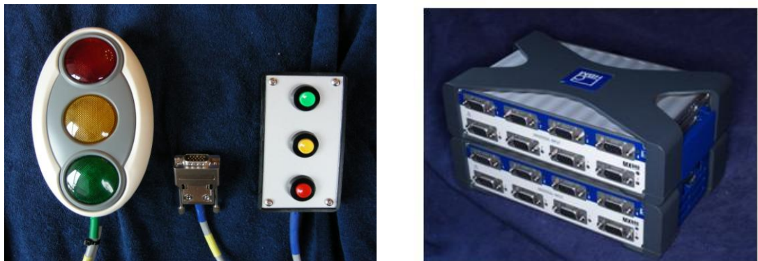
Figure 9. Ad hoc three-light warning system generator and HBM-MX 840 interface for sincronization (© Ing. M. Balestra)
