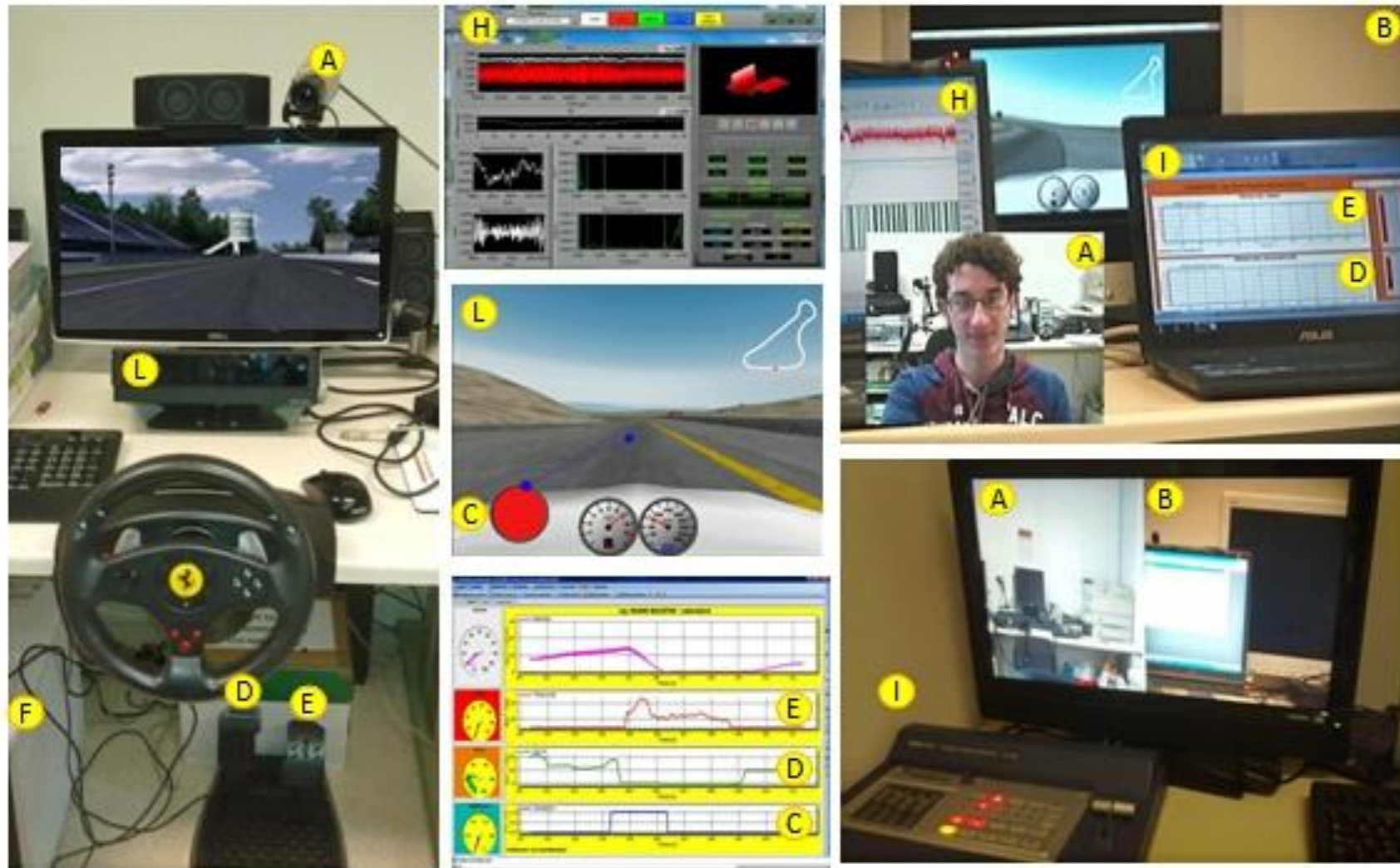
Figure 34. TPRCS setting: A-B) HD Cameras; C) Stimuli generator; D) U-93 sensor run of the accelerator pedal (mm, 100 Hz); E) WA-300 sensor, pressure on the brake (N, 100 Hz); F) Signal interface MX-840; H) BIOPAC SYSTEM MP100 + MindWare HRV 3.0.17, EDA 3.0.15; I) Control panel for synchronization HBM+MB; L) Tobii X120 Eye Tracker.
