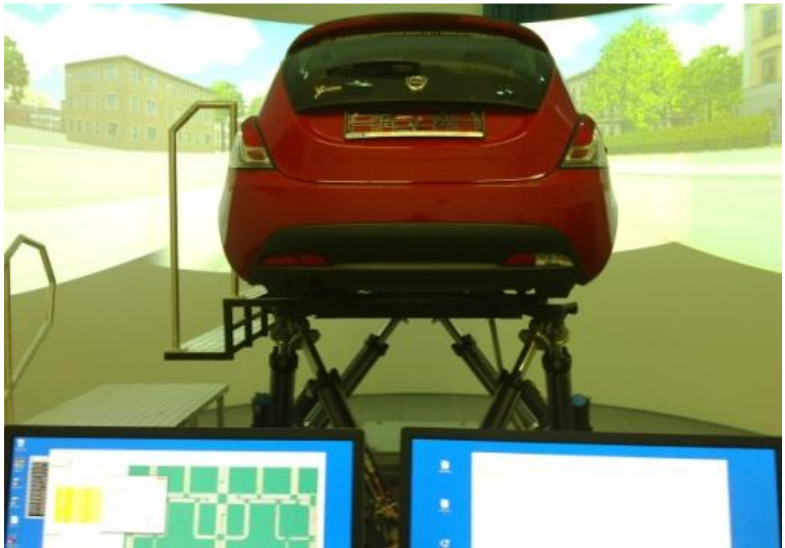
Figure 57. Driving simulator used for this third studio. It was an AutoSim (Norway), consisting of a full vehicle cabin (Lancia Ypsilon) installed on a 6 axes Stewart platform, and programmed by Prof. Virga and Vangi of the Florence University, IT
