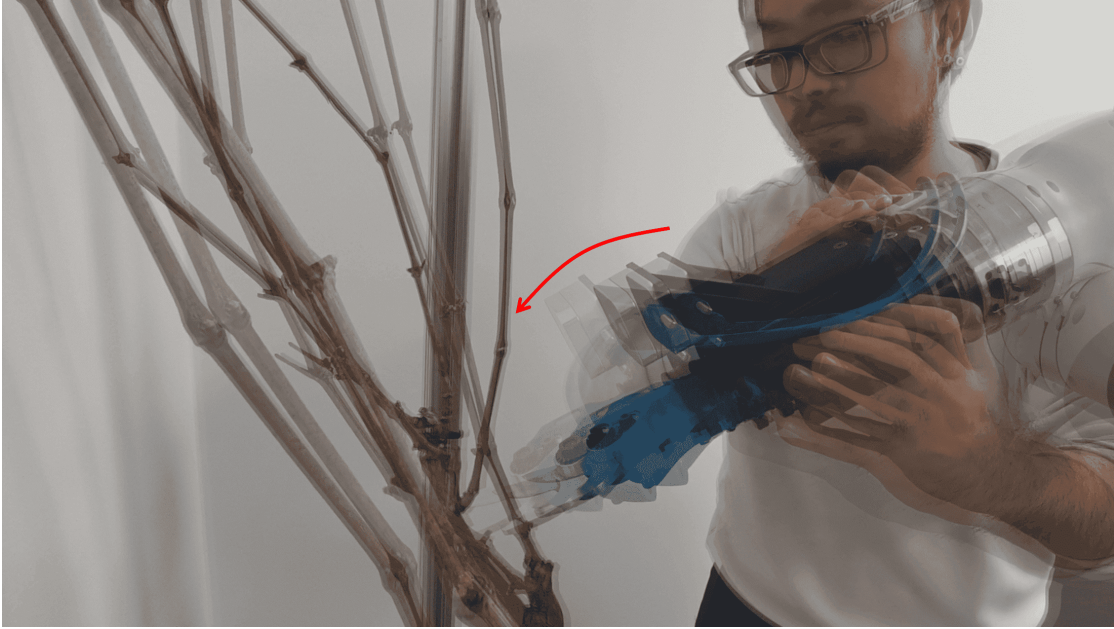
Figure 6.3: Demonstration of pruning robot, in which Cartesian position trajectories of end-effector and force profile are recorded. The red arrow indicates the movement process of the robot.
